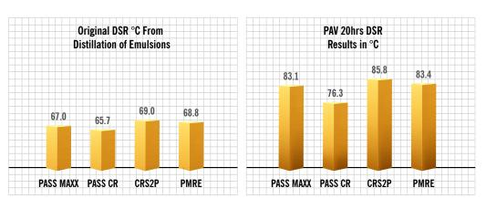
AFTER 20 HOURS IN THE PRESSURE AGING VESSEL (PAV) THE BINDER AGES AND BECOMES MORE VISCOUS AFTER MODERATE AGING.
