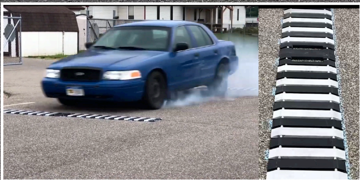
NO MOVEMENT in the SKID TESTING
