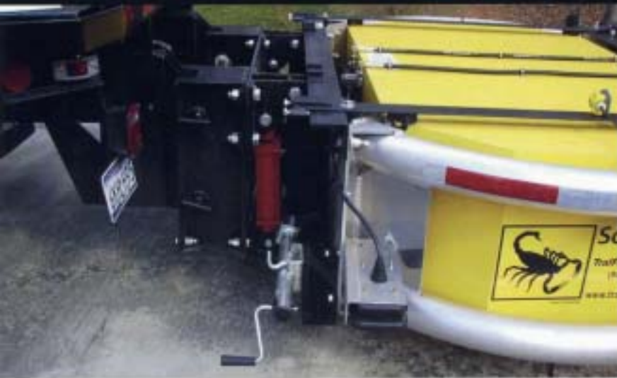
Scorpion TMA attached to a truck using a 12" Extension Frame and Back-up Assembly.
