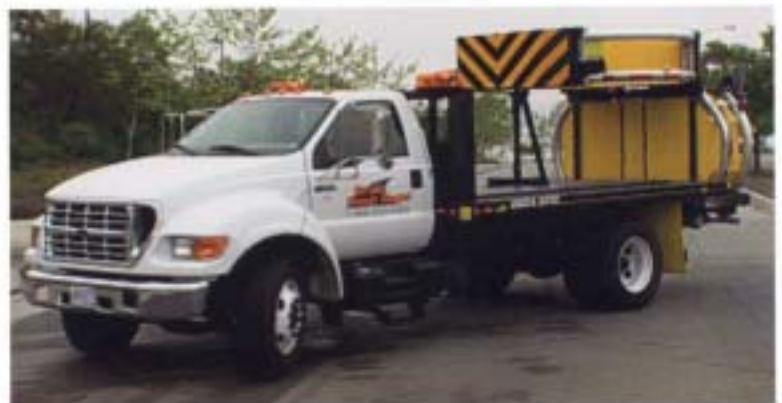
Scorpion's compact design and minimal 3' rear overhang, reduces the chance of hitting fences, signposts and other objects while backing-up or turning corners.
