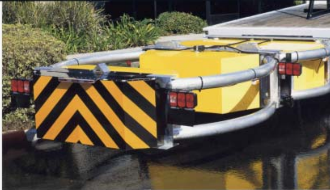
The Scorpion TMA is hydraulically powered and measures 13 feet long when fully extended, making it ideal for stationary and mobile construction zones.
