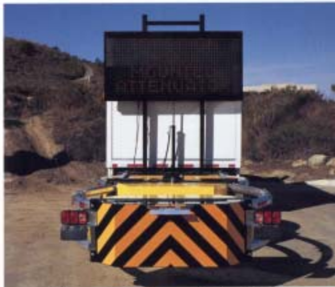
Rear view of the Scorpion TMA with message panel in the raised position, ready for use on the job site. The bottom of the message panel when elevated, is 7' above the surface of the roadway, in full compliance with Federal Standards.
